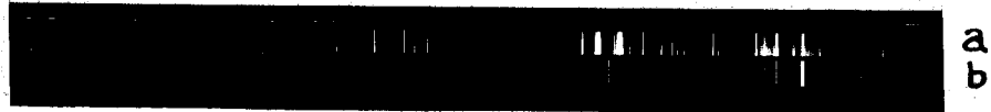
Figure 1. (a) Copper arc in sulfur vapor. (b) The explosion of magnesium with copper sulfate.
